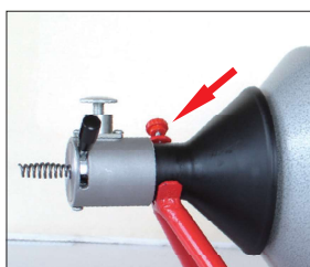
Insert the hand held complete machine to the relevant clip position and lock the screw properly
