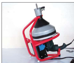
The dredging and cleaning operation can be carried out with two different angles of the frame
