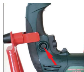
Adjust the electric drill to the appropriate rotation speed before using and push down the locking press button to hold the electric drill switch on the normally open position.
