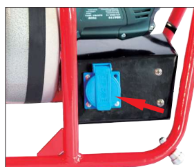
Insert the power supply cord plug of the electric drill into the supply socket on the frame. Connect the power plug on the frame with the socket power reliably.
